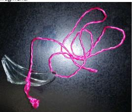
6. Weigh the glass fragment suspended in water to the nearest 0.01 g and record this value. Convert this value to milliliters. (Recall that 1g of water has avolume of 1 mL.) This is the volume of the glass sample.
